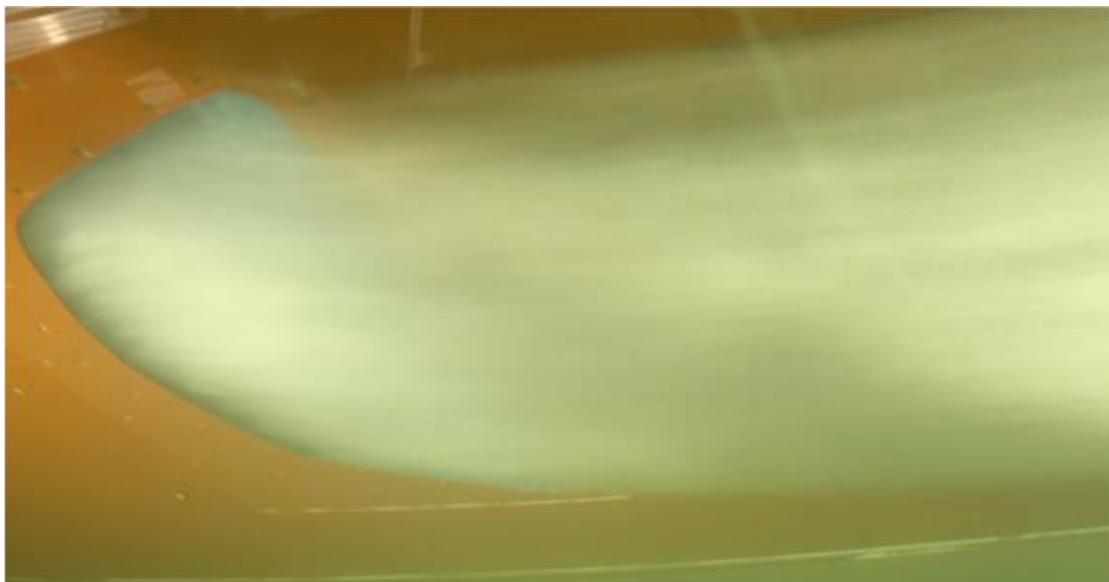
Fig 9: Air bubbles being injected during HyKaT experiments
