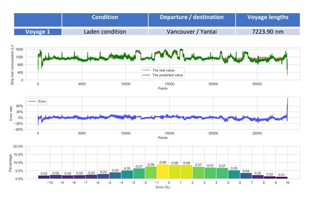
The ship digital twin can accurately capture ship energy system for ship fuel consumption in real conditions
