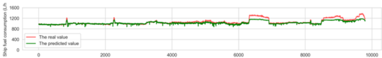
Figure 4: Comparison of fuel consumption from predicted (green line) and real (red line) data.
